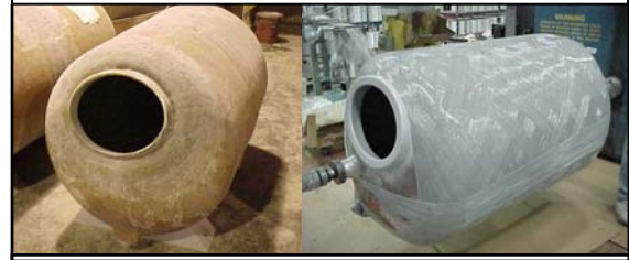
Dual Construction Method: Shell & Winding
